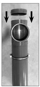
Fasten the extension piece with the agglutinated t-piece and cap at the wall bracket and adjust the direction. The distance from the middle of the t-piece to the floor should be at least 1 meter (compare schematics at page 3).
