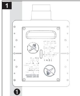
Attach the frame of the inlet to the stud (2x4) Make sure that the inlet is leveled (figure 1) and that you leave 8 cm free behind the inlet.
